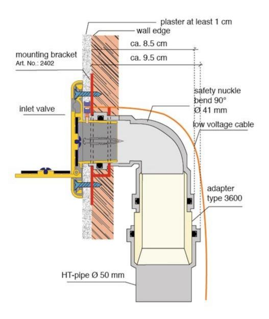
Installation example with safety knuckle bend, 41 mm (item no. 2501) using the adapter, type 3600 with the 90° safety knuckle bend and the BVC-PP pipes, 50 mm dia for walls < 12 cm.
